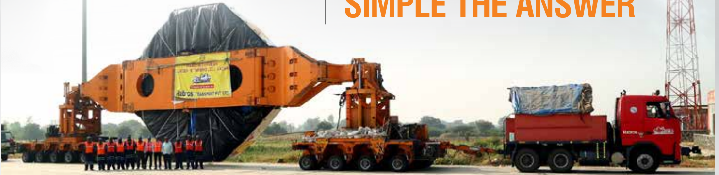
END SHIELD movement from L&T Hazira to RAPP, Rawatbhata using specially designed Rotatiting fixture to overcome en route bottlenecks Size: 9.5 m x 9.4 m x 1.70 m • Weight: 120 MT + 65 MT(Fixture)
