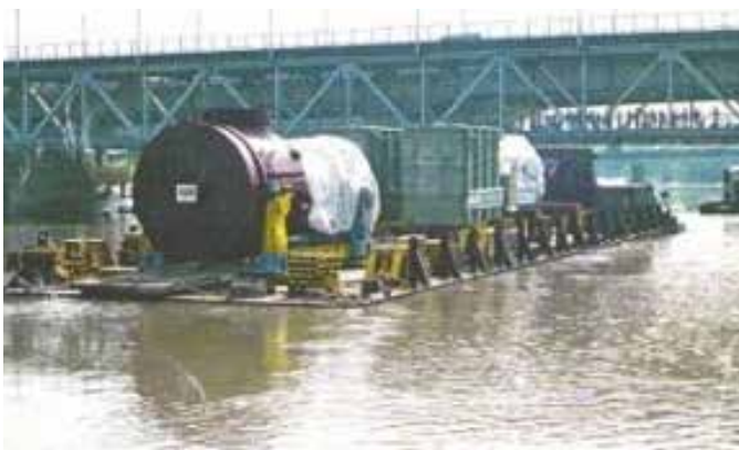
Barging of a Gasturbine, Generator and Transformers to the Connaught Bridge Power Station (1991)
