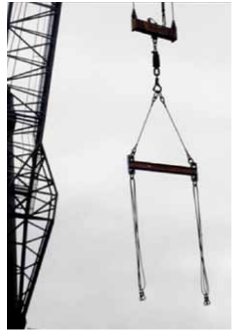
Fig.14 Typical lift beam, incorrect design
