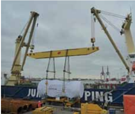
Fig.12 A combination of Lift- and spreader beams
