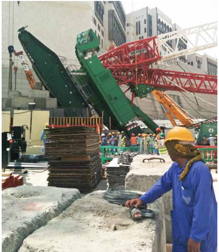
Fig.03 Blown over Liebherr LR11350 in Mecca
