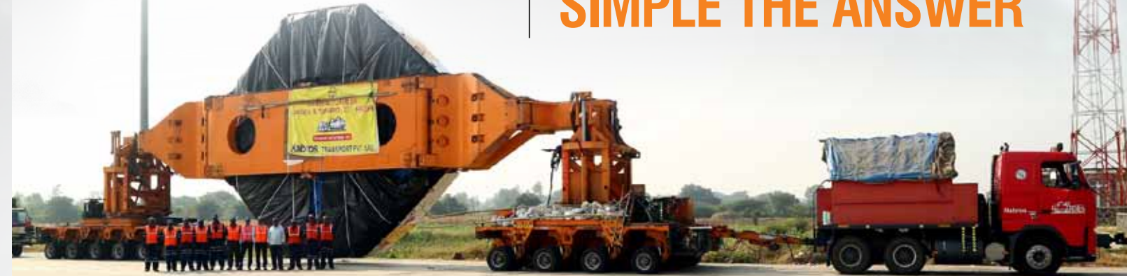
END SHIELD movement from L&T Hazira to RAPP, Rawatbhata using specially designed Rotating fixture to overcome en route bottlenecks Size: 9.5 m x 9.4 m x 1.70 m • Weight: 120 MT + 65 MT(Fixture)
